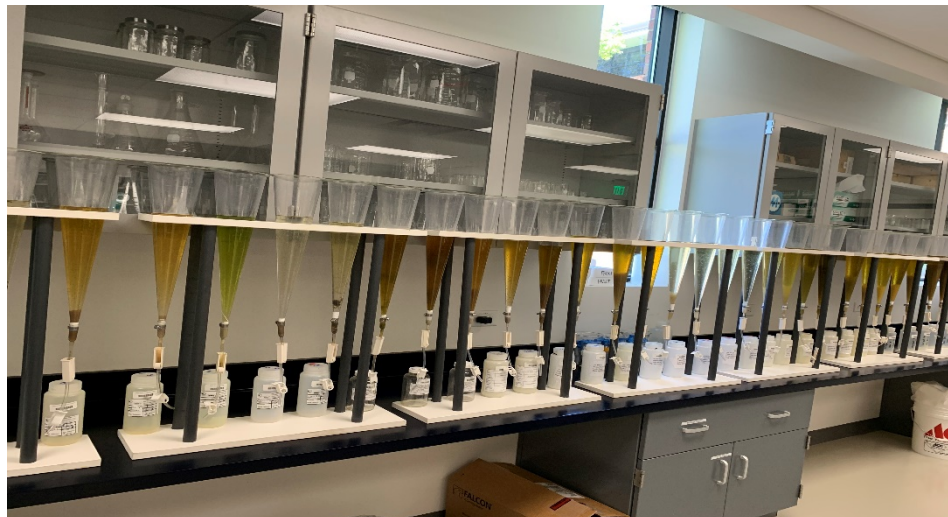
Figure 3 Samples settling in Imhoff cones prior to analysis
