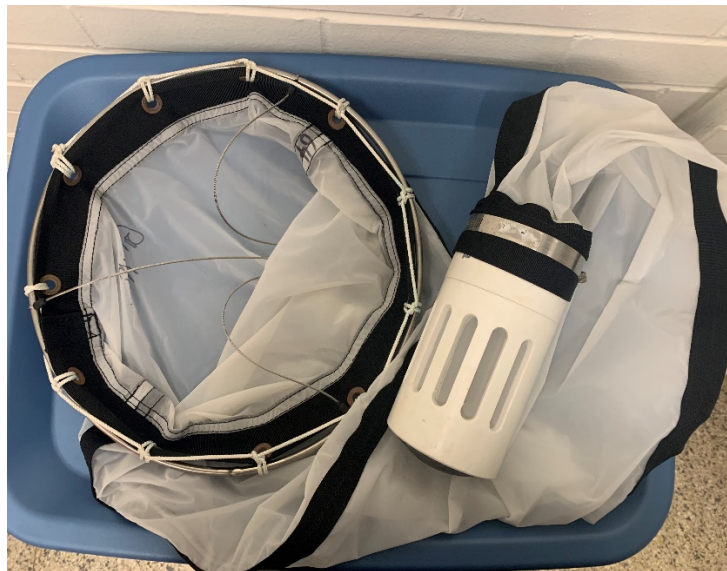
Figure 1 Plankton tow net with attached cod end
